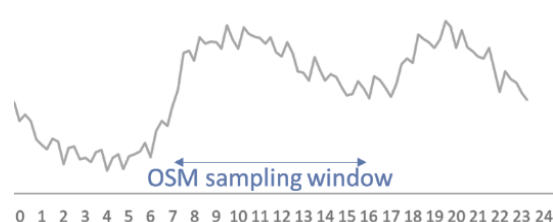
24-hr pattern of treated sewage discharge
