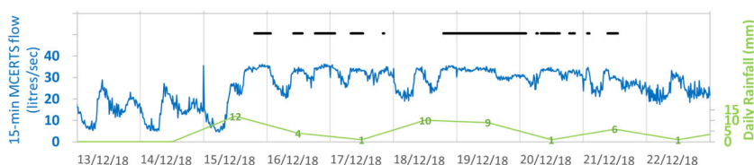
Fig. 1 WWTP1: example effluent flow pattern for 10 days annotated with EDM confirmed spilling intervals. A 24-h (midnight to midnight) daily flow pattern of 96 15-min-interval average flow rates (litres/second) of treated effluent is shown in blue. The black horizontal, linear annotations represent EDM recorded intervals denoting a discharge from a storm tank (i.e., consented spill or potentially unconsented spill of untreated sewage), the shortest being 15 min and the longest over 24-h. Total daily rainfall (mm/d) is provided in green. The first two days, with no detected spills, show diurnal patterns of low flow between midnight (previous day) and the first peak after mid-morning, followed by a lull until a second, smaller peak in the evening. The next seven days (15/12/18 through 21/12/18) involve spill intervals of various length (black EDM line), showing a flattening of flow, which is typical of storm discharge during heavy rainfall. The last day shows elevated flows and a partial return to a diurnal flow pattern with no spills reported.
